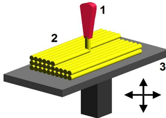
**1 – Nozzle ejecting molten plastomer, 2 – deposited material (modelled part), 3 – controlled movable table.**
